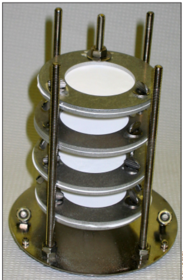
Figure 1 Polar Organic Chemical Integrative Sampler (POIS) housing with four sorbents. Source: https://www.cerc.usgs.gov/pubs/center/pdffdocs/pocis.pdf , 3/16/2022
